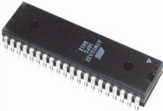
A microcontroller is a small computer on a single integrated circuit containing a processor core, memory and programmable input/output peripherals.
