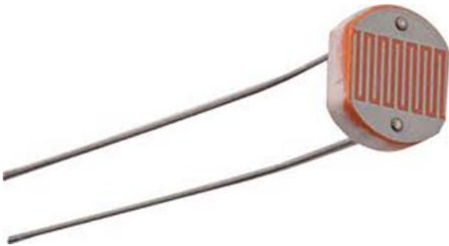
One of the features of an optical sensor is its ability to measure the changes from one or more light beams. This change is most often based around alterations to the intensity of the light. When a phase change occurs, the light sensor acts as a photoelectric trigger, either increasing or decreasing the electrical output, depending on the type of sensor.
