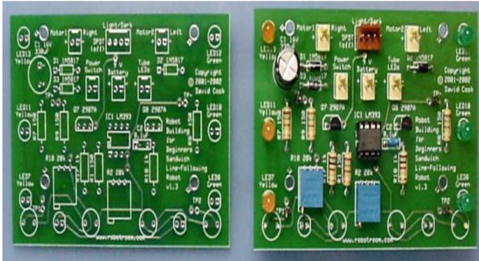
Before a PCB can be physically fabricated it has to be decide where all the components will be placed and arranged and how the PCB traces will connect the different components. This process is called PCB design.
