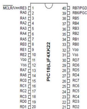
For this project we are using a 40-pin PIC18LF45K22 Microcontroller which is a PIC type Microcontroller. PIC is a family of
