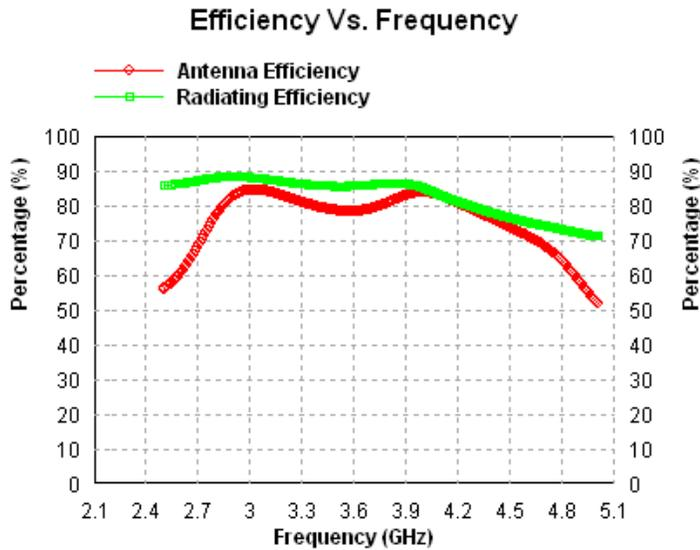
Fig. 4: Variation of Efficiency with frequency for proposed antenna design
