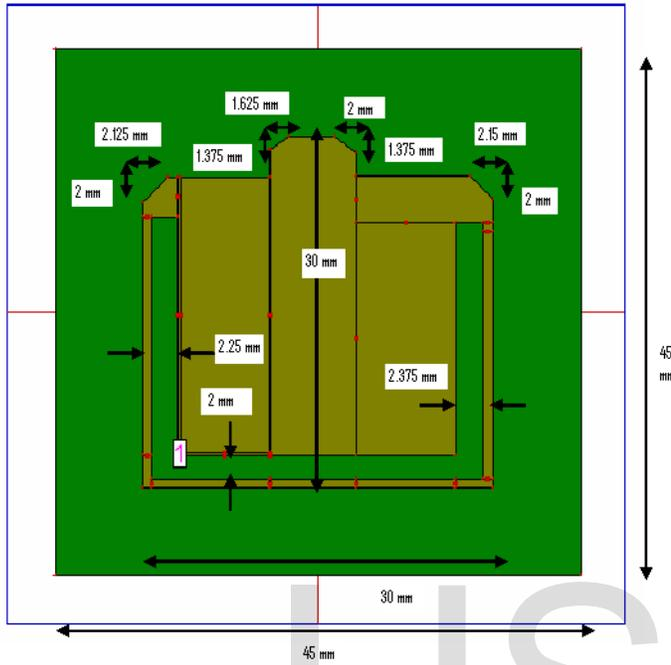
**Fig. 1: Modified square microstrip patch antenna with finite ground plane**
