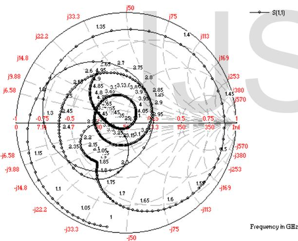
Fig. 5: Impedance loci for proposed antenna design
