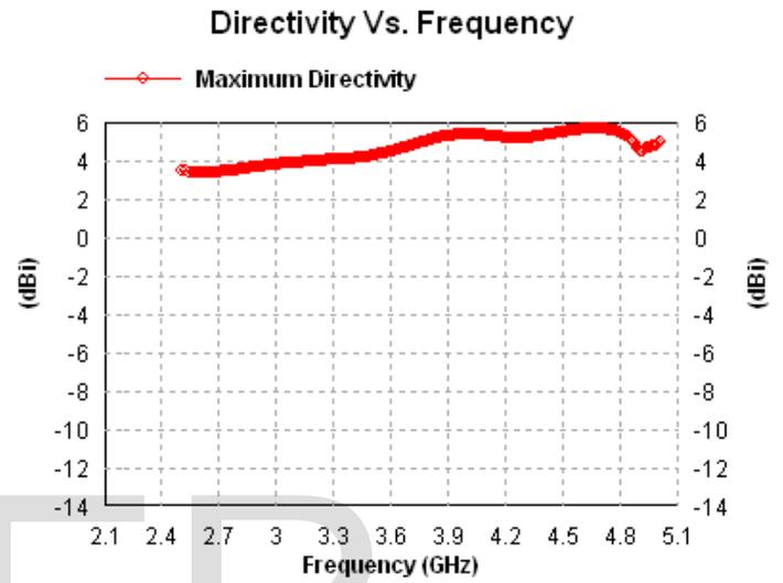
**Fig. 3: Variation of directivity with frequency for proposed antenna design**
