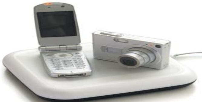
A Splash power mat uses induction to recharge multiple devices simultaneously.
