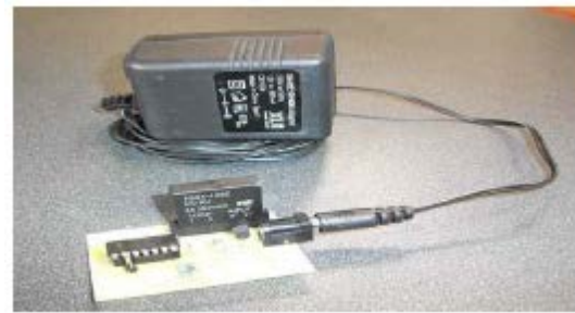
Figure 8: Fabricated relay control unit
