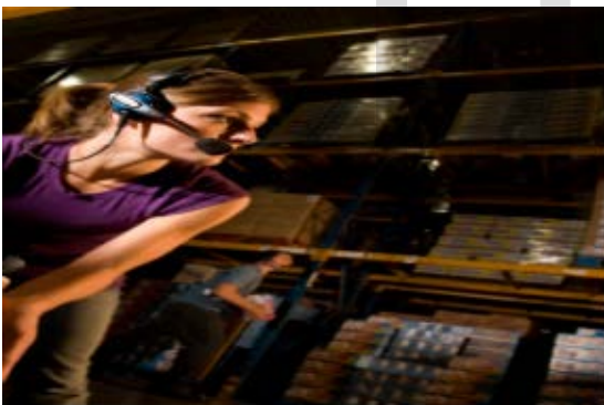
Fig 4 :voice enabled wearable computer that guides the worker in picking up the right objects from the right counters and shelves[10]
