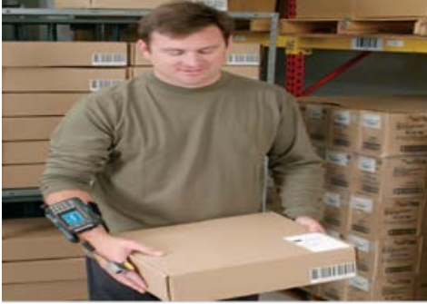
Fig 3:A Ring scanner with wrist mounted wearable computer that frees the both hands of the worker while scanning the products [9]
