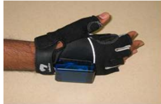
Fig2: iGlove with RFID reader that gives information about what item the user is touching with his hand [5]
