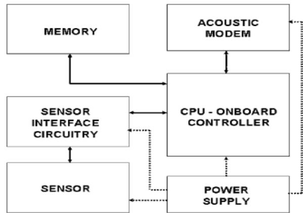
Fig. 3. Internal architecture of an underwater sensor node.
