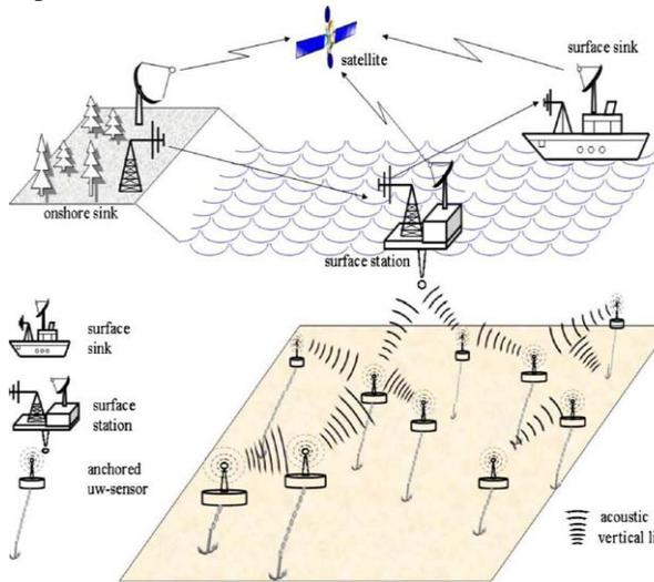
Fig. 5. Architecture for 3D underwater sensor networks.
