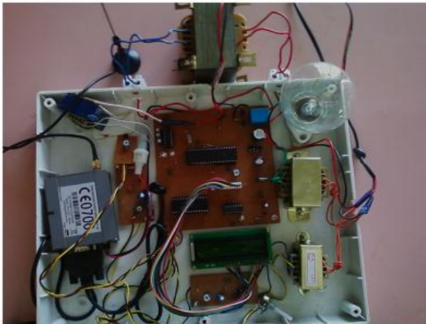
Fig.6. Prototype model of microcontroller based transformer health condition monitoring kit.
