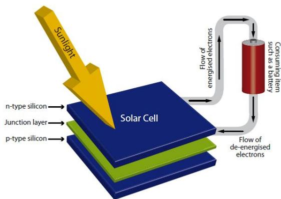
Fig.1:Principle of operation of a PV Cell.
