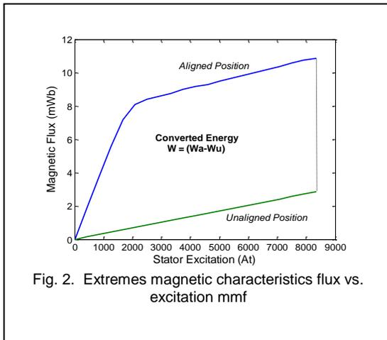
Fig. 2. Extremes magnetic characteristics flux vs. excitation mmf
