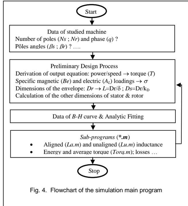
Fig. 4. Flowchart of the simulation main program
