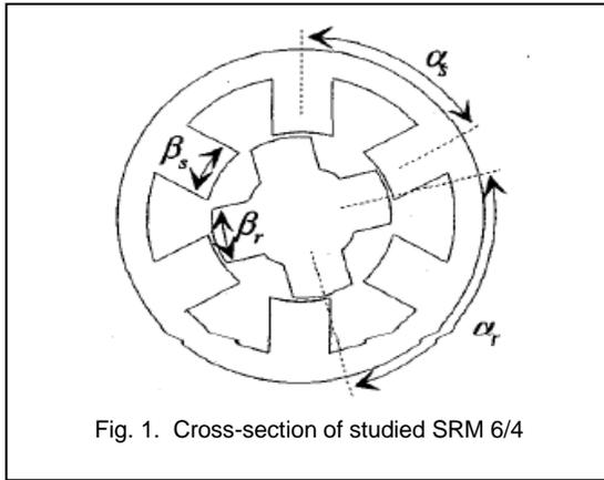
Fig. 1. Cross-section of studied SRM 6/4
