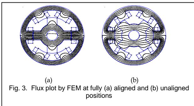
Fig. 3. Flux plot by FEM at fully (a) aligned and (b) unaligned positions
