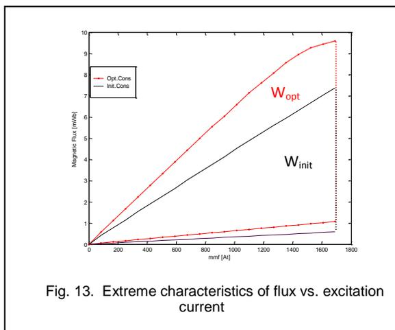
Fig. 13. Extreme characteristics of flux vs. excitation current
