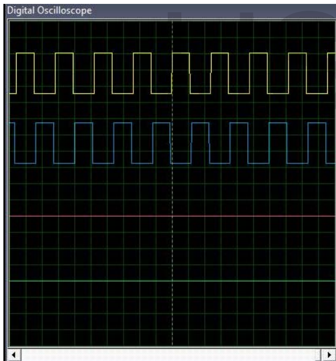
Fig.c2: inverter input signals waveform
