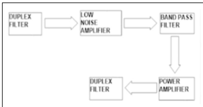
Fig. 3. Block Diagram of Signal Amplifier
