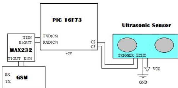
until when the echo of the sound waves echoed back to the sensor. The ECHO pin which is being connected to the C3 pin of the PIC16F73 microcontroller is continuously monitored to detect its status. The timer1 of the microcontroller is used for the purpose of calculating the time period for the sound wave to travel back to the sensor. Then, the calculated time can be computed through the following equation into the distance (cm) unit.
