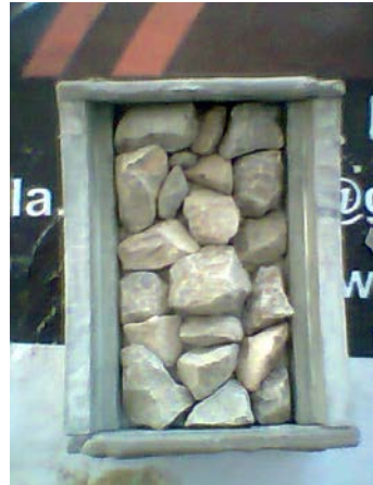
Figure 4. Aggregates placement in Mould
