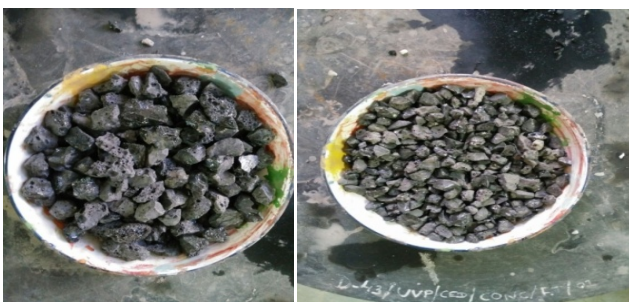
Fig.2. Cupola Slag crushed to 20mm and 10mm
