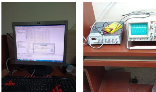
Fig.7- Porting digital values of a triangular wave through FPGA(Left)and DAC output(Right)
