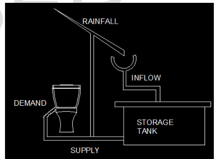
Fig. 1. Configuration of the rainwater harvesting system
