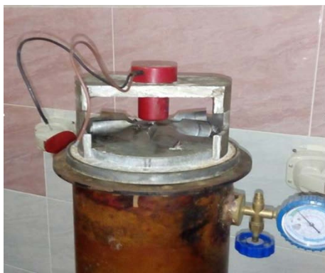
Fig.5 Photo of turbine and electric generator configuration
