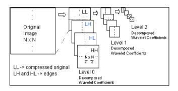
Figure 1: A 3 level Wavelet Decomposition of N x N image
