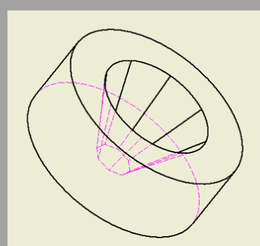
Fig. 11. Streamlined die for extrusion of octagonal section
