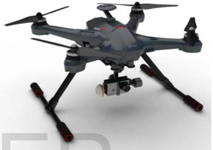
Fig. 2. Quadcopter drone with its landing skids.
