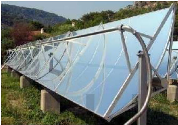
Fig. 1: Solar parabolic trough with porous receiver
