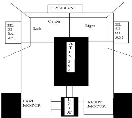
Fig 11.A Pictographic representation of the vehicle
