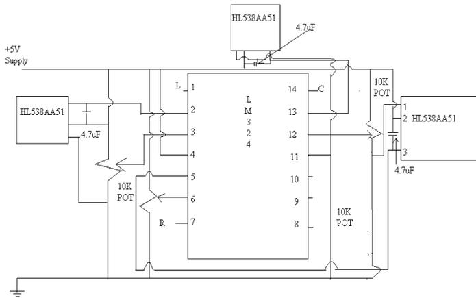
Fig 5. IR sensor and comparator circuit
