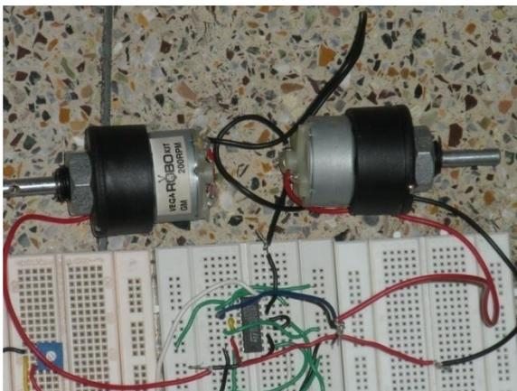
Fig 10.A picture of our entire circuit consisting of the three sensors, one comparator, microcontroller and driver
