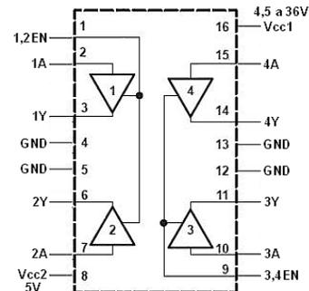
Fig 3. Internal circuit of L293D
