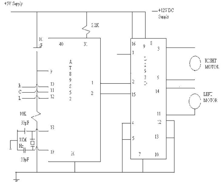
Fig 6. Microcontroller and driver circuit
