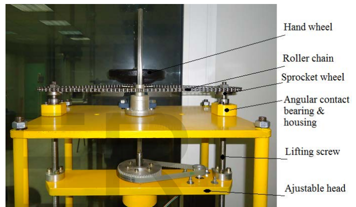
Fig. 6: Height adjustment mechanism
