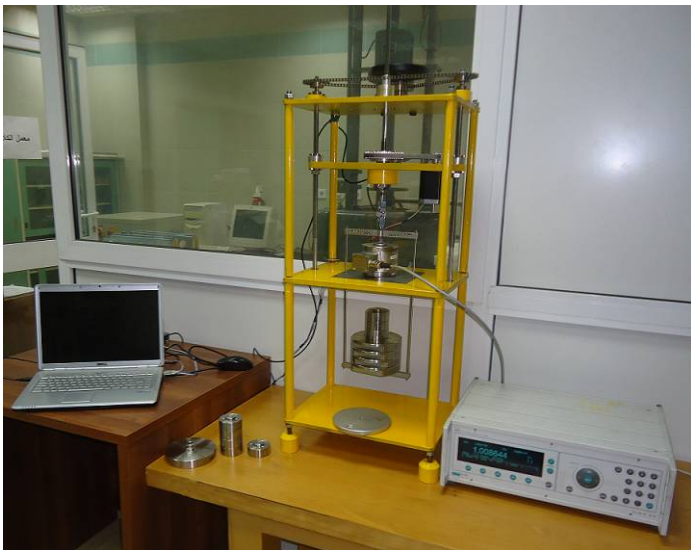
Fig. 2: The new 200 N force standard machine
