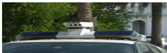
Figure 2.2.1 The Dubai police use three Petards ANPR cameras to monitor vehicles in front and either side of the patrol car
