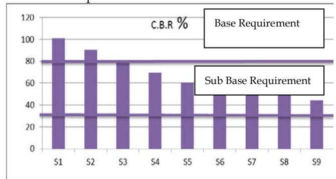
Figure 8: CBR Values for different mixes
