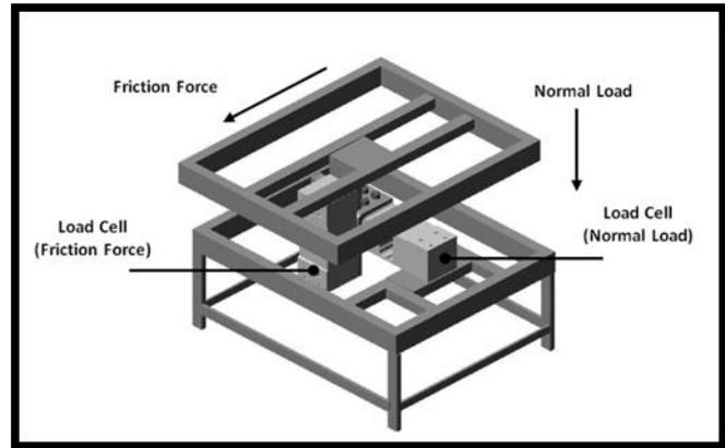
Fig. 1 Details of the test rig.
