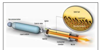
Fig. 1. Describes the combustion process,here the solid fuel is vapourized as a result of heat transferred from flame zone to fuel grain.
