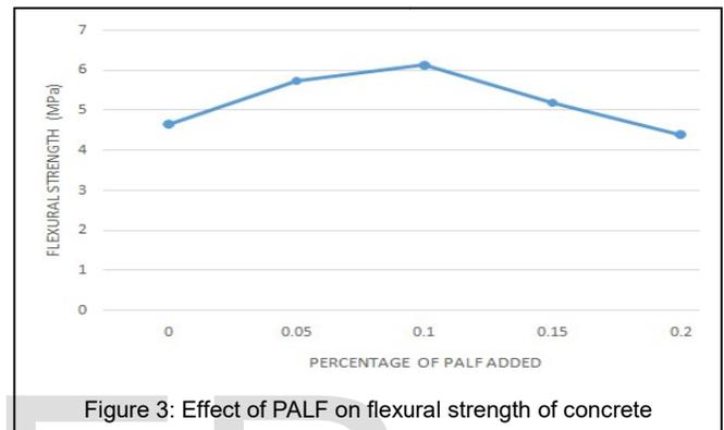
Figure 3: Effect of PALF on flexural strength of concrete
