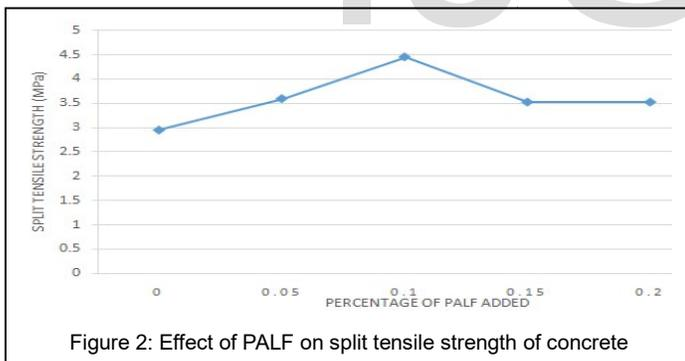
Figure 2: Effect of PALF on split tensile strength of concrete
