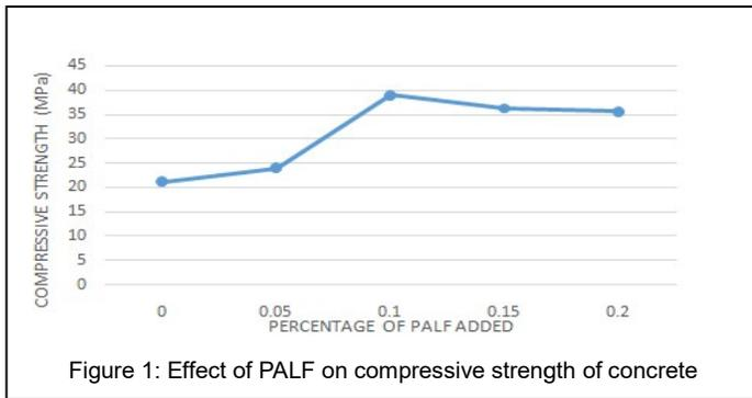
Figure 1: Effect of PALF on compressive strength of concrete
