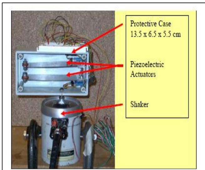
To demonstrate the power harvesting advantage, 40 and 80 mAhr Nickel Metal Hydride batteries are recharged with each individual actuator then charged with both actuators connected in parallel. For a 1.4 Hz frequency (a brisk walking pace), the parallel combination charges two 40 mAhr batteries in 3.09 hours, and two 80 mAhr batteries in 5.64 hours. The individual actuators require 16.1
