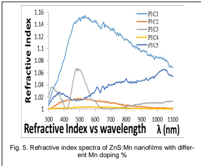
Fig. 5. Refractive index spectra of ZnS:Mn nanofilms with different Mn doping %
