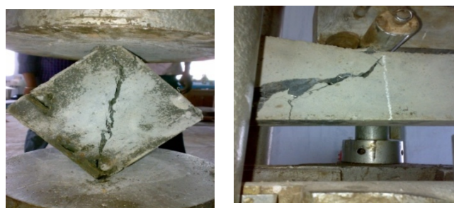
Fig.1 Diagonally placed tesile failure
