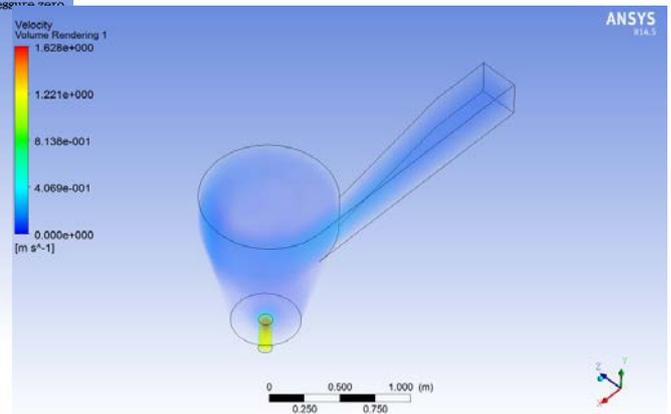
Figure.10 Velocity distribution for 100 mm Outlet diameter
