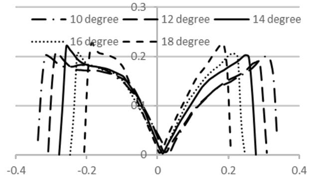
Figure.3 Tangential velocity distribution along the line drawn at 0.1 meters from bottom face for different cone angle.
