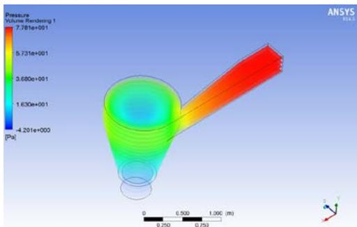
Figure. 8 Pressure distribution for 400 mm outlet diameter
