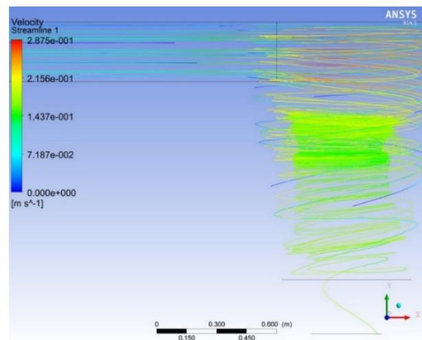
Figure.5 Stream lines with base plate.
