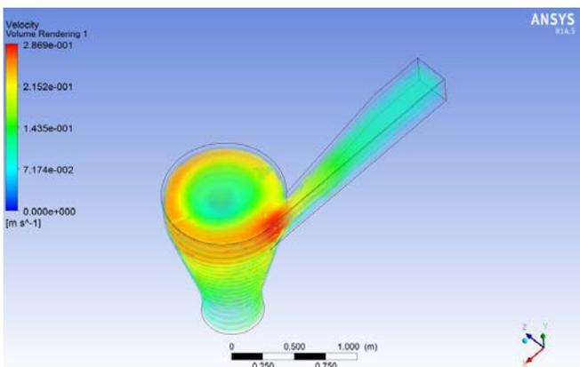
Figure.9 Velocity distribution for 500mm Outlet diameter
