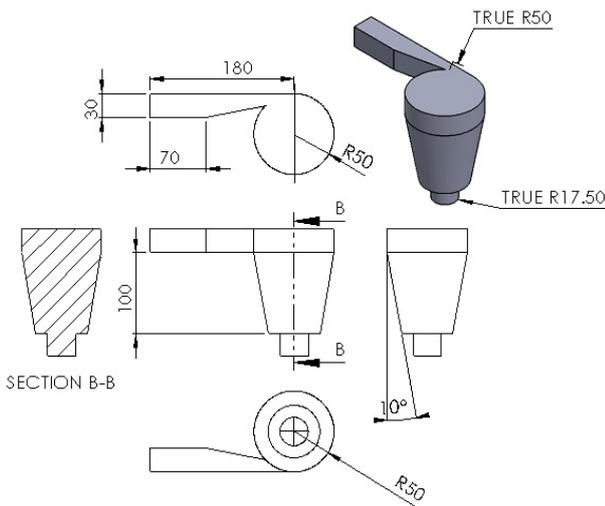
Figure.1 Dimensions of the basin and runner
