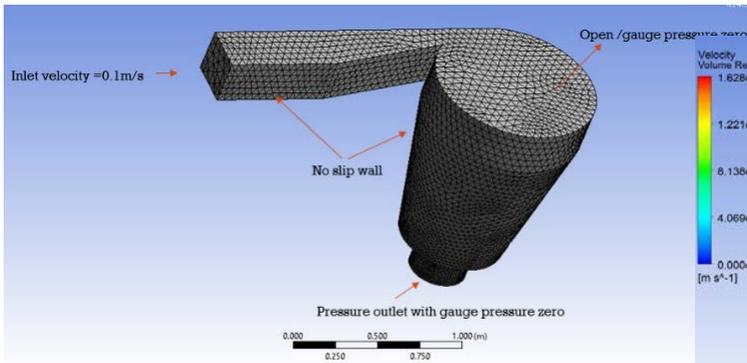
Figure.7 Meshed model with boundary conditions
