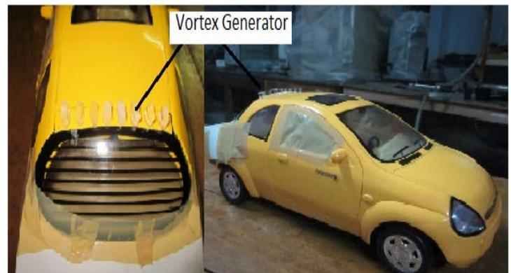
Fig 4. Experimental model of car with vortex generator
