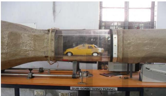
Fig 5. Experimental Setup of Car model with Vortex generator under sub sonic Wind tunnel
