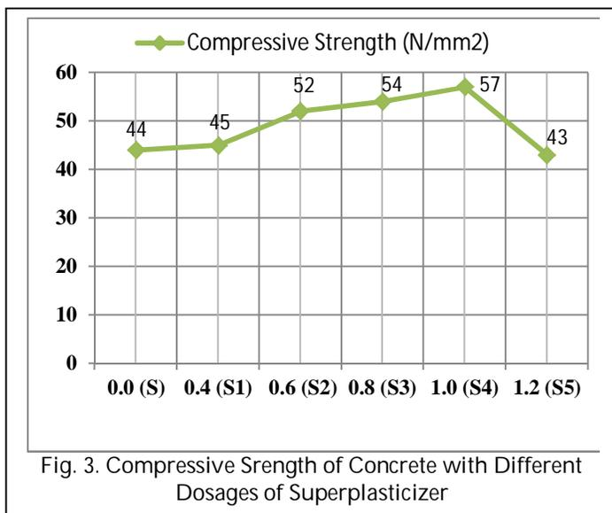
Fig. 3. Compressive Strength of Concrete with Different Dosages of Superplasticizer
