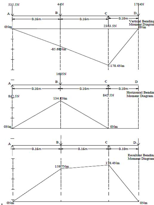
**Fig. 12: Bending moment diagrams for the main roller shaft**
