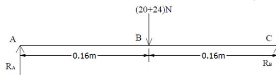
**Fig. 14: Vertical loading of the driven roller shaft (Point Load)**
