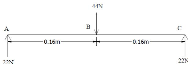
**Fig. 15: Vertical bending moment of the driven roller shaft**
