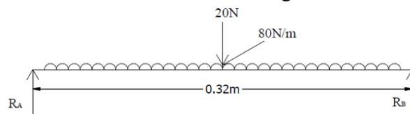
**Fig. 13: Vertical loading of the driven roller shaft (Uniformly Distributed Load)**
