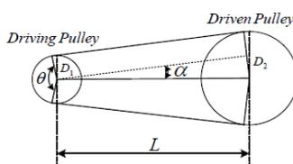
**Fig. 11: Belt geometry of the electric motor and main roller shaft pulley (Khurmi and Gupta, 2005).**
