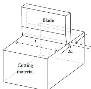
**Fig. 2: Interaction between the blade and the material while cutting** (Zhou *et al.*, 2006)
