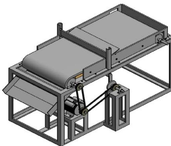
**Fig. 10 : Isometric view of the slicer**
