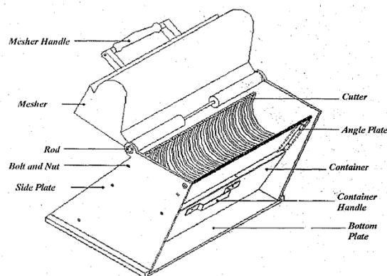
**Fig.5:Mechanized plantain slicer** (Obeng, 2004)
