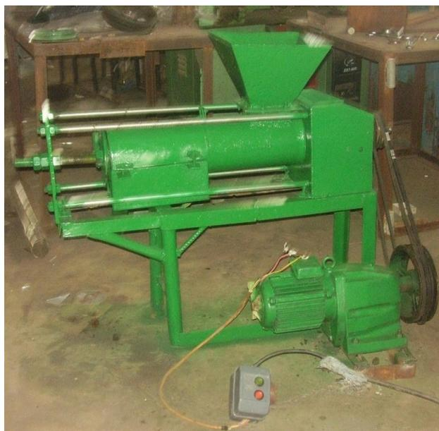
Figure 2: Palm oil screw press developed
