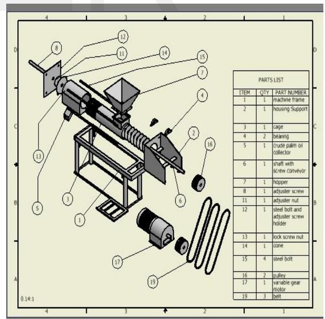
Figure 1: Exploded view of the palm oil screw press showing the component parts
