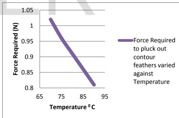
Fig. 3. A graph of force required to plucking out down feather against temperature
