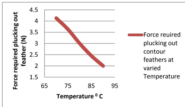
Fig. 2. Showing a graph of force required to plucking out contour feather against temperature
