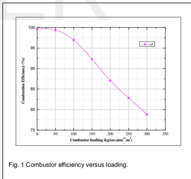
Fig. 1 Combustor efficiency versus loading.
