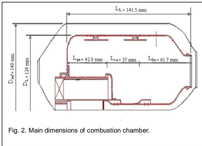
Fig. 2. Main dimensions of combustion chamber.
