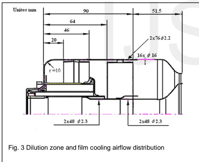
Fig. 3 Dilution zone and film cooling airflow distribution
