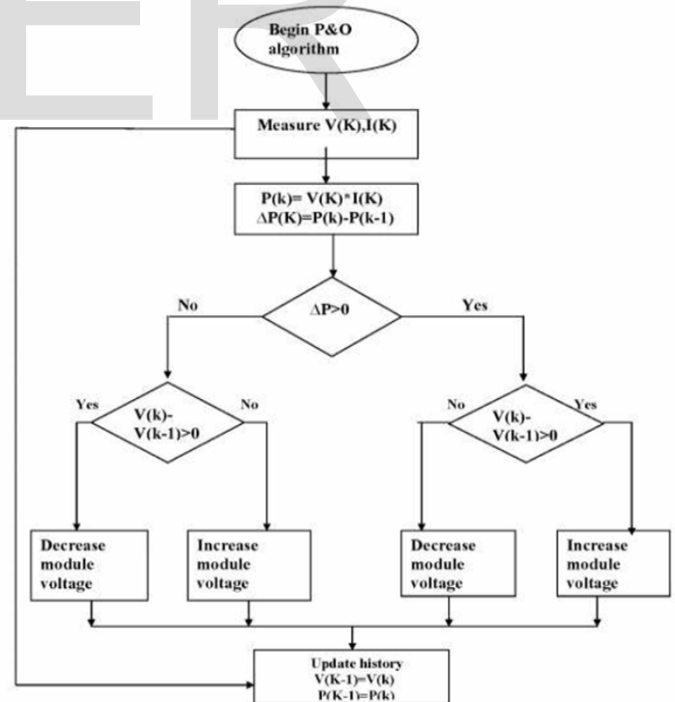
Fig.4 Perturb and observe (P&O) algorithm flow chart
