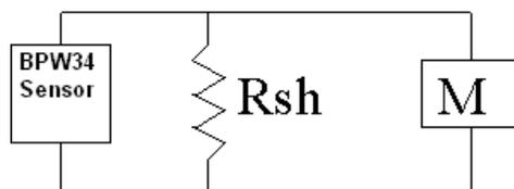
At a full sunlight output current of 3.4 mA current is obtained by the sensor. Thus by applying ohms law.
