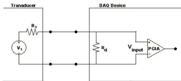
Figure 1.-Model of a Typical Transducer and DAQ Device
