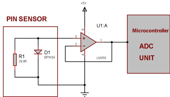
Figure: Unity gain Buffer for the ADC to decrease the source impedance here LM358 is used as a unity gain buffer , PIN photodiode BPW34 solar irradiance sensor, R1 as shunt resistor
