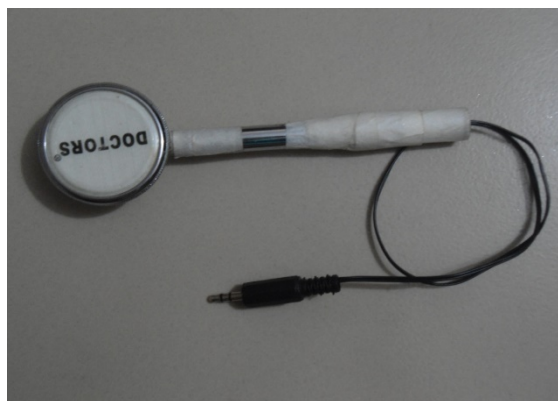
Fig 14: Implementation of chest piece for auscultation.
