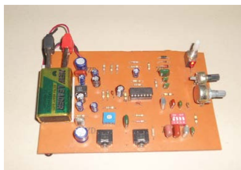
Fig 15: Implementation of amplifier circuit with features in PCB board.
