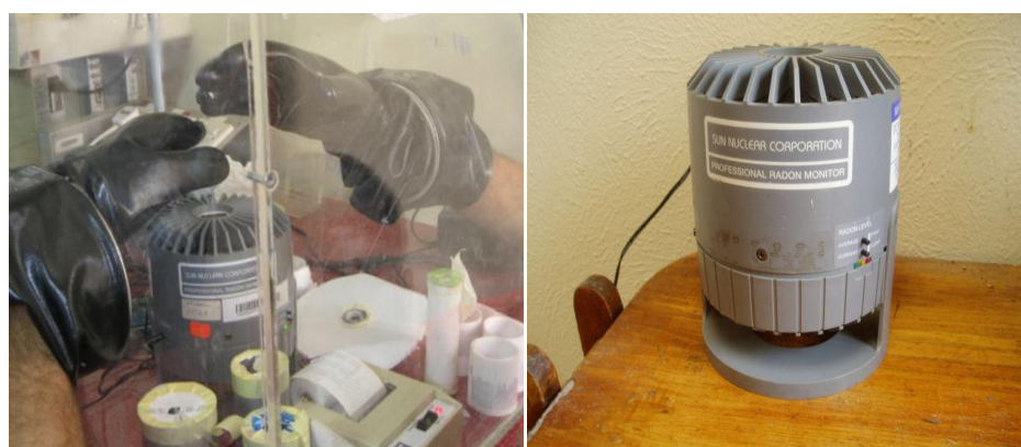
Fig. 1. The radon chamber and the continuous radon monitor model (1023)
