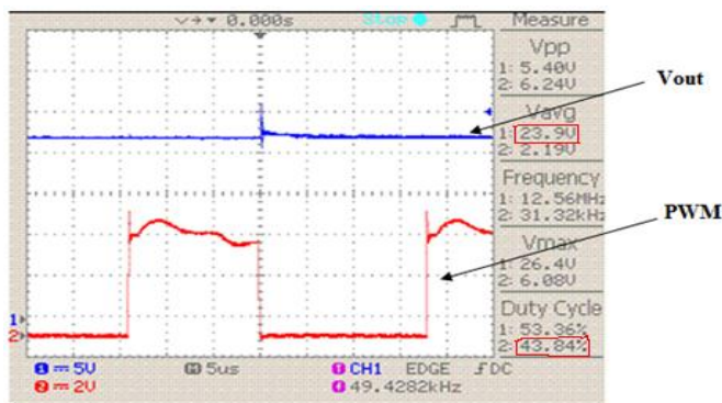
Figure 19 output of boost converter when input voltage is 13.6V and duty cycle is 43% and input current 0.3 A with output voltage of microcontroller as 3.0V.
