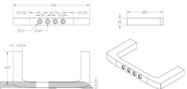
Fig 7: Design of Bumper Beam
