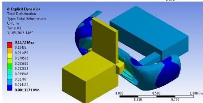
Fig 11: Simulation graphic of Low Speed Impact Test
