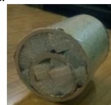
Fig 5: Double cylinder filled with foam
