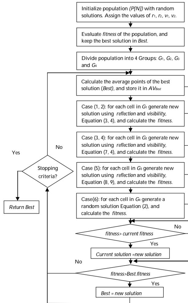
Fig. 7. General principle of CFA
