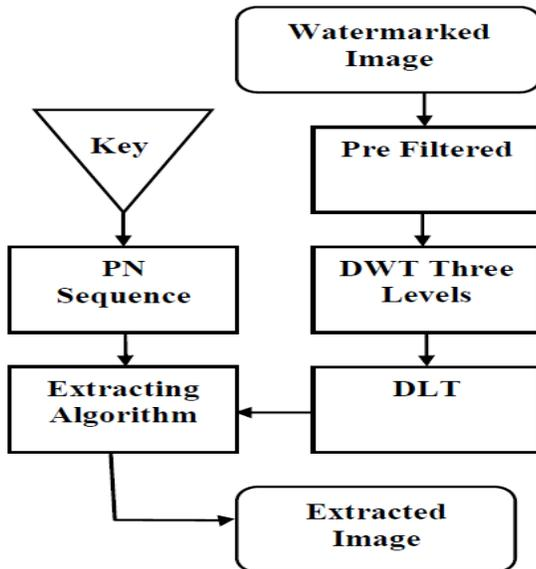
Figure - 7 The Combined DWT and DLT Extracting Algorithm
