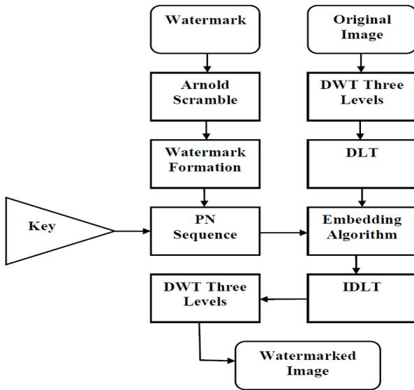
Figure - 4 The Combined DWT and DLT Embedding Algorithm
