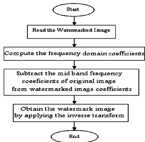
Figure - 3 The Watermark Detection Flowcharts
