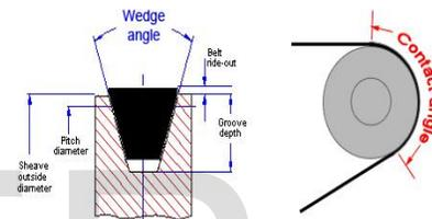
fig 2 - Dimensions Of V-Belt
