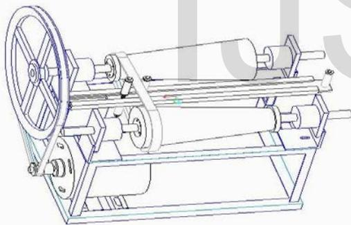
fig7 .Setup of Cone CVT
