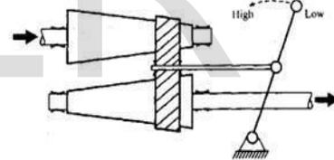
fig5.Belt and Lever mechanism
