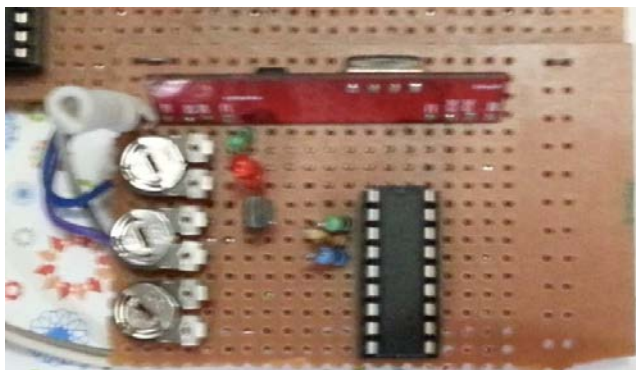
fig 10. RF receiver implemented on PCB
