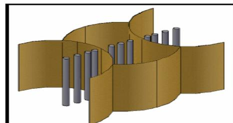
Fig 3 installing internal short pile
