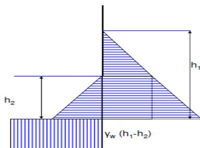
The maximum probable height outside the cofferdam during construction and the water height inside the cofferdam during various stages of construction need to be considered. These result in the net design pressure.
