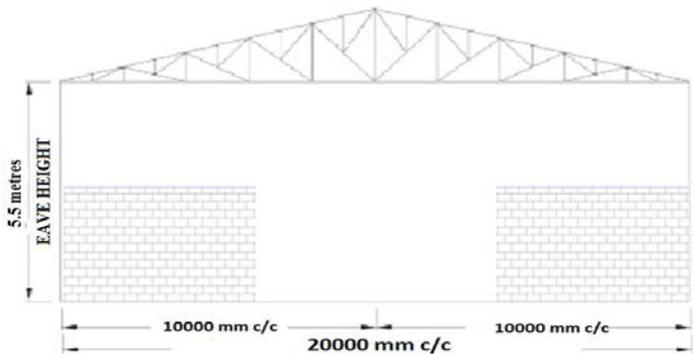
Fig.2 Single Frame of a Conventional Steel Building
